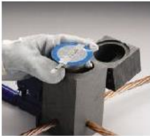
Step 1 Insert CADWELD PLUS package into mold.
